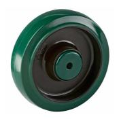
standard Wheel with roller bearing and elastic rubber tyre with hardness 70  $^{\circ}$  shore A on polyamide
