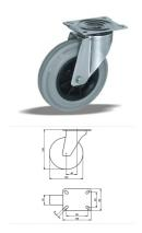
stainless steel Swivel castor with an overall height of 128 mm Wheel diameter x width: 100 x 32 mm Top plate with 4 mounting holes of 9 mm, mounting hole distance 80x60 mm and top plate outer dimensions: 105x85 mm Wheel with plain bearing and grey rubber tyre with hardness 83 ° shore A on polypropylene.
