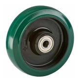
stainless steel Wheel with ball bearing and elastic rubber tyre with hardness 70 ° Shore A on polyamide Wheel diameter x width: 125 x 35 mm Axle hole: 12 mm Hub length: 44 mm
