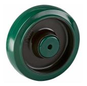
stainless steel Wheel with roller bearing and elastic rubber tyre with hardness 70 ° Shore A on polyamide Wheel diameter x width: 125 x 35 mm Axle hole: 12 mm Hub length: 44 mm
