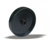
standard Wheel with plain bearing and solid polyamide wheel with hardness 70±5 Shore D Wheel diameter x width: 80 x 35 mm Axle hole: 12 mm Hub length: 44 mm
