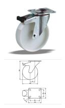
standard Swivel castor with brake with an overall height of 128 mm Wheel diameter x width: 100 x 35 mm Top plate with 4 mounting holes of 9 mm, mounting hole distance 80x60 mm and top plate outer dimensions: 105x85 mm Wheel with plain bearing and solid polyamide wheel with hardness 70±5 Shore D the double brake system, brakes the turning of the wheel and the swivel rotation.
