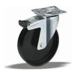
standard Swivel castor with brake with an overall height of 128 mm Wheel diameter x width: 100 x 38 mm Top plate with 4 mounting holes of 9 mm, mounting hole distance 80x60 mm and top plate outer dimensions: 105x85 mm Wheel with ball bearing and solid polyamide wheel with hardness 70±5 Shore D the double brake system, brakes the turning of the wheel and the swivel rotation.
