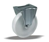
standard Fixed castor with an overall height of 128 mm Wheel diameter x width: 100 x 35 mm Top plate with 4 mounting holes of 9 mm, mounting hole distance 80x60 mm and top plate outer dimensions: 105x85 mm Wheel with ball bearing and solid polyamide wheel with hardness 70±5 Shore D.
