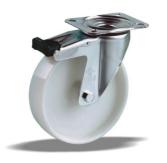
standard Swivel castor with brake with an overall height of 155 mm Wheel diameter x width: 125 x 35 mm Top plate with 4 mounting holes of 9 mm, mounting hole distance 80x60 mm and top plate outer dimensions: 105x85 mm Wheel with ball bearing and solid polyamide wheel with hardness 70±5 Shore D the double brake system, brakes the turning of the wheel and the swivel rotation.
