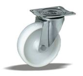
standard Swivel castor with an overall height of 155 mm Wheel diameter x width: 125 x 38 mm Top plate with 4 mounting holes of 9 mm, mounting hole distance 80x60 mm and top plate outer dimensions: 105x85 mm Wheel with ball bearing and solid polyamide wheel with hardness 70±5 Shore D.
