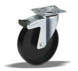
standard Swivel castor with brake with an overall height of 155 mm Wheel diameter x width: 125 x 35 mm Top plate with 4 mounting holes of 9 mm, mounting hole distance 80x60 mm and top plate outer dimensions: 105x85 mm Wheel with ball bearing and solid polypropylene wheel with hardness 70±5 Shore D the double brake system, brakes the turning of the wheel and the swivel rotation.
