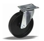
standard Swivel castor with an overall height of 155 mm Wheel diameter x width: 125 x 38 mm Top plate with 4 mounting holes of 9 mm, mounting hole distance 80x60 mm and top plate outer dimensions: 105x85 mm Wheel with ball bearing and solid polyamide wheel with hardness 70±5 Shore D.
