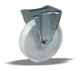
standard Fixed castor with an overall height of 155 mm Wheel diameter x width: 125 x 38 mm Top plate with 4 mounting holes of 9 mm, mounting hole distance 80x60 mm and top plate outer dimensions: 105x85 mm Wheel with ball bearing and solid polyamide wheel with hardness 70±5 Shore D.
