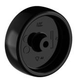
furniture Wheel with plain bearing and solid polypropylene wheel with hardness 60±5 ° Shore D
