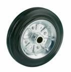
standard Wheel with plain bearing and black rubber tyre with hardness 80 ° Shore A on steel rim with electrogalvanization zinc plating anti-corrosion protection Cr6-free Wheel diameter x width: 125 x 37 mm Axle hole: 15 mm Hub length: 44 mm
