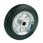
standard Wheel with roller bearing and black rubber tyre with hardness 80 ° Shore A on steel rim with electrogalvanization zinc plating anti-corrosion protection Cr6-free Wheel diameter x width: 125 x 37 mm Axle hole: 15 mm Hub length: 44 mm
