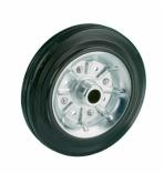
standard Wheel with roller bearing and black rubber tyre with hardness 80 ° Shore A on steel rim with electrogalvanization zinc plating anti-corrosion protection Cr6-free
