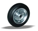
standard Wheel with ball bearing and black rubber tyre with hardness 80 ° Shore A on steel rim with electrogalvanization zinc plating anti-corrosion protection Cr6-free
