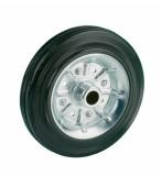
standard Wheel with plain bearing and black rubber tyre with hardness 80 ° Shore A on steel rim with electrogalvanization zinc plating anti-corrosion protection Cr6-free
